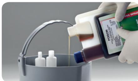
**7.** Unscrew and remove the red cap. Pour the solution from the dispensing cup into the full Pulse Cleaner. Take care to not allow more solution from the main bottle flow into the dispensing cup.
