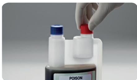
**3.** Slightly unscrew the red cap (i.e. 1 – 2 revolutions), but do not completely unscrew it.
